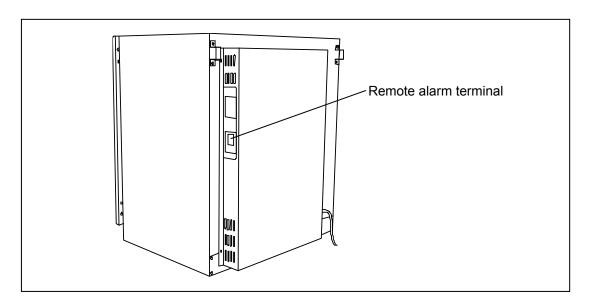
The remote alarm terminal is a contact output.
